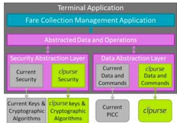
**Figure 4-3 Terminal Application structure after CIPURSE V2 integration**
